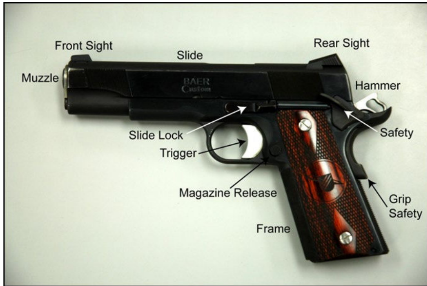
Figure 12.23: Parts of the 1911 series semi-automatic pistol
