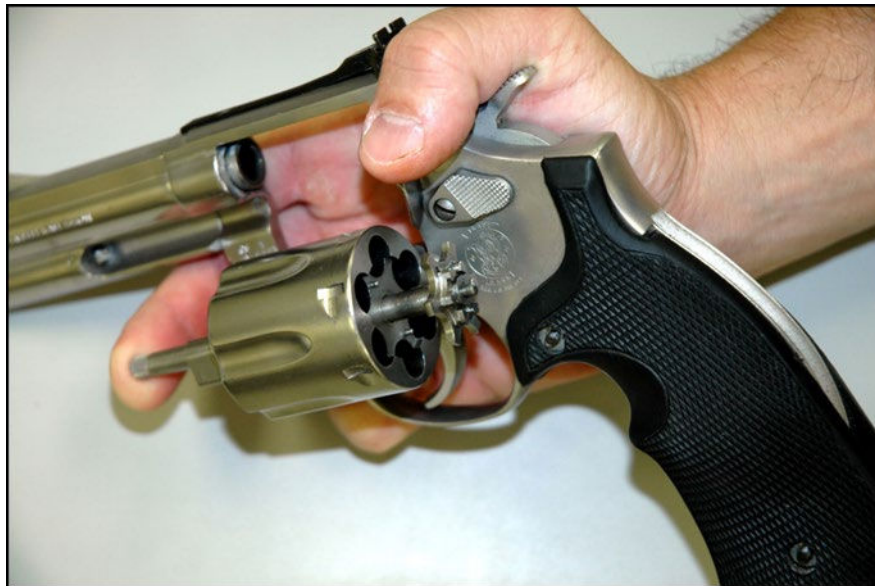
Figure 12.16: Chambers and extractor
