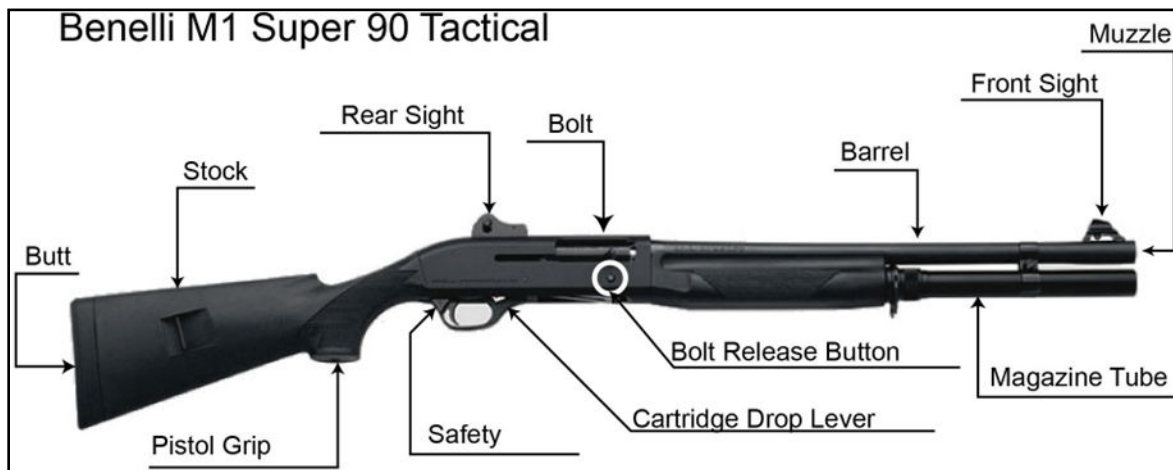
Figure 12.27: Parts of the Benelli M1 Super 90 shotgun
